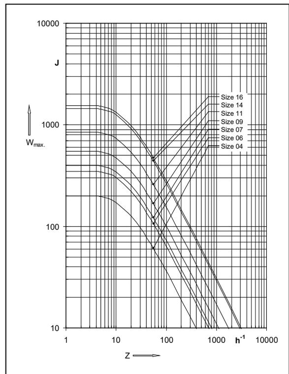
Fig. 38/1: Max. switching work W<sub>max</sub> per switching operation as a function of the number of switching operations per hour Z (values based on n=3000 rpm; applicable to dynamic brakes)
