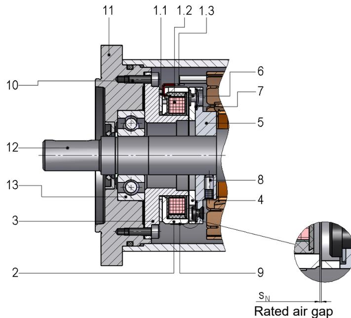
Fig. 13/1: Permanent-magnet single-face brake 86 621..H00 with armature 300
