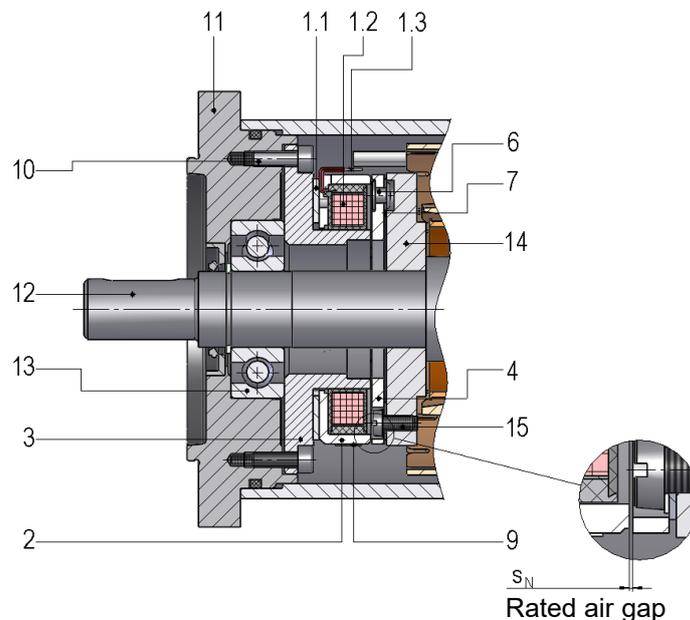
Fig. 12/1: Permanent-magnet single-face brake 86 621..H00 with armature 200
